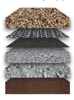
**40mm Resiscape Resin Bound surface course**, (approximately 5mm incorporated into the Reinforced Plastic Matting), hand applied and trowelled as per the Resiscape installation guide.
